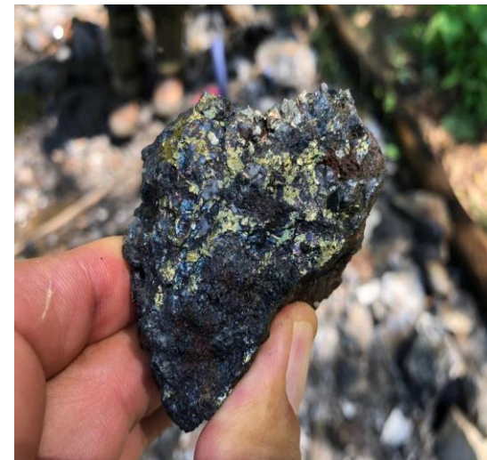
Crystals and massive chalcopyrite and galena in a sample of polymictic breccia
