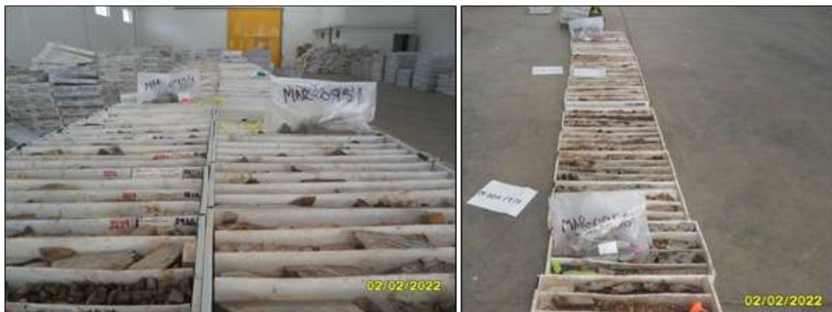
Figure 12.6 Verification Core Samples from Diamond Drilling Holes Collected During the 2022 Site Visit
