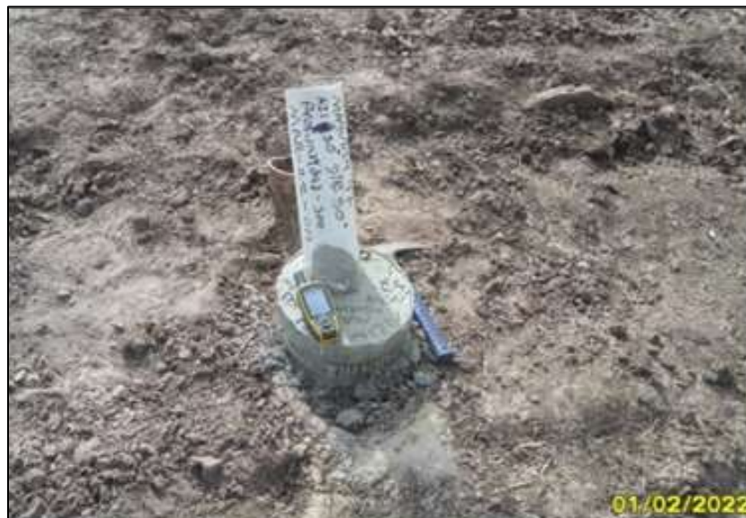
Figure 10.3 Collar Monuments for the Drill Holes Completed by Magna
