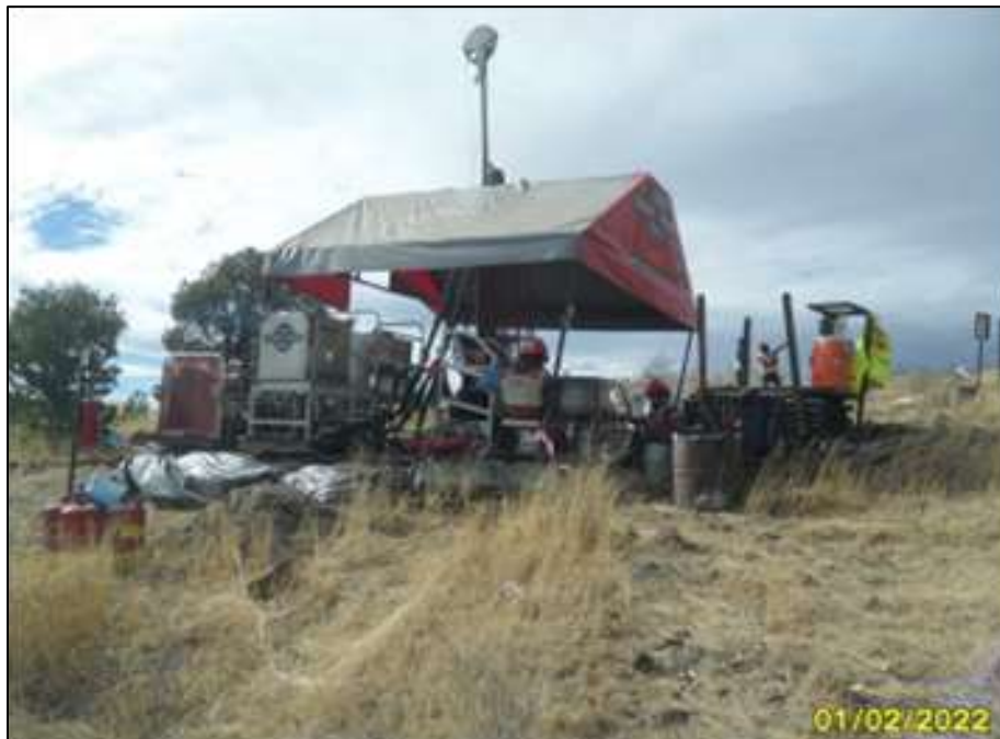
Figure 10.2 Portable Diamond Drill Hole Rig used during the 2021-2022 Campaign
