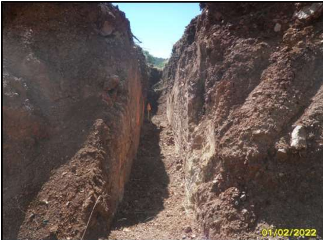
Figure 9.5 Surface Exploration Trench across the Mineralized Vein
